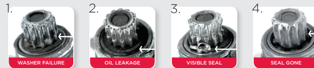
1. Washer failure and oil leakage. 2. Oil leakage. 3. Seal failure / visible seal. Indents due to worn socket. 4. Seal gone / visible ball bearings. Rounded teeth due to removing container while running.
