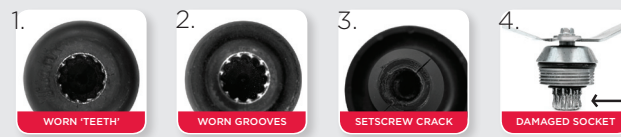
1. Worn 'teeth' due to removing container while running. 2. Worn grooves due to placing container on motor base without centering pad or touching container while machine is running. 3. Cracking at setscrew due to over tightened screw or due to a foreign object in the container. 4. Drive socket or blade assembly needs to be replaced.
