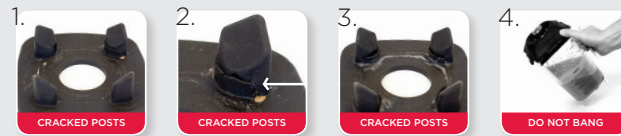
Tearing at container posts due to banging container on counter or improper cleaning of centering pad (placing pad in dishwasher or using improper cleaning or sanitizing products).
