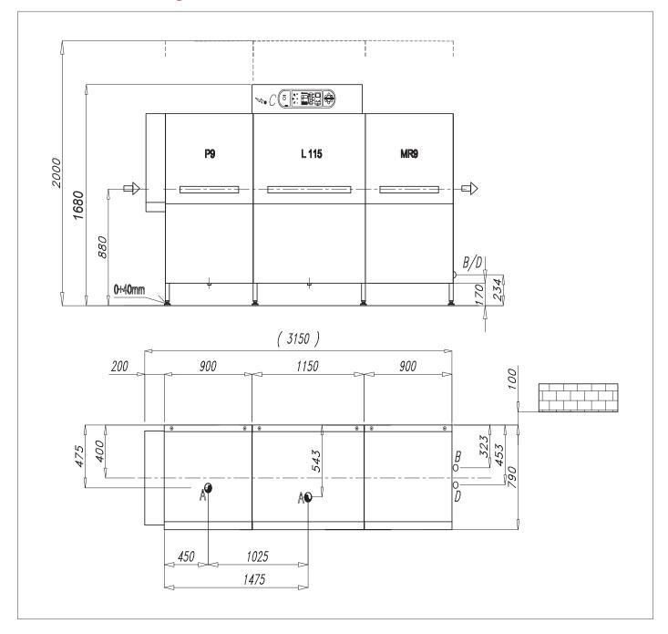
The drawing refers to the standard machine with no optional - Feeding direction: left  $/\ \mbox{right}$
