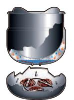
Cleveland steam jacketed kettles offer ultra efficient heat transfer, uniform heating and superior product handling. Steam jacketed kettles offer faster cooking times because two thirds of the cooking surface comes into contact with the product at a much lower temperature, compared to stock pots that use a much higher temperature only at the bottom of the pot. In addition, accurate
