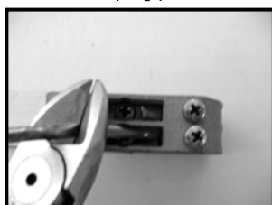
Pull wires taut using a pair of pliers and a vice and screw the wires down on the clamping plate.
