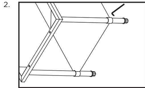
Use 4 x 8mm Allen key screws to secure the shelf section to the legs.
