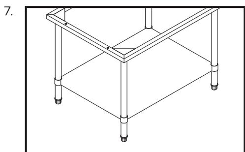
Level the stand by adjusting the adjustable feet on the bottom of the stand.
