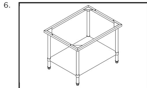
Locate top and ensure it is correctly aligned and inter-locks with the stand.
