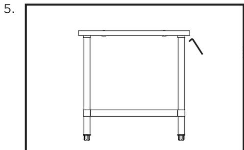
Use 4 x 8mm Allen key screws to secure bench-top section to the legs.
