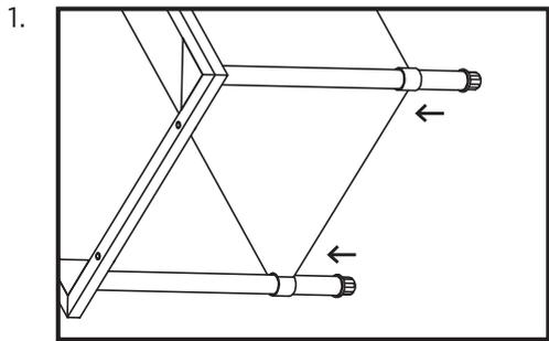
Insert legs through the bottom of the shelf. Locate the scribed mark and position bottom of shelf on the scribe mark.
