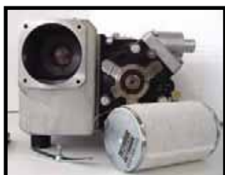
Remove tensioner and filter from the housing
