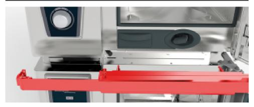
Combi-Duo table-top appliances 6 x 1/1 GN, 6 x 2/1 GN, 10 x 1/1 GN and 10 x 2/1 GN: To change the air filter on the top Combi-Duo appliance, please open the doors of both units and pull forward the cover plate. Watch out for the USB cable and the hose for the door drip pan. This will give you free access to the air filter so you can replace it as described above.
