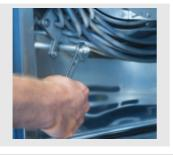
Loosen the union nut on the moisturing nozzle (turn anti-clockwise – spanner size 15).
