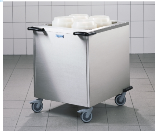
Platform stacker BDUH/60-60/4-S (heated by circulating air). Adjustable crockery column guide by rods, 4 of which are supplied as standard. It can be easily adapted to suit all current crockery sizes between for example Ø 170 mm and Ø 280 mm by special base grid with 7 x 7 = 49 locations.
